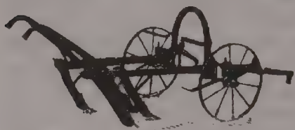
Fig. 147. A tongueless walking cultivator with wooden gangs.
