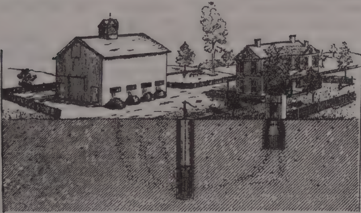
Fig. 300. A sketch showing how the water of a shallow well may become contaminated from manure yards and cesspools. (Kansas Exp. Sta. Bul. 143.)
