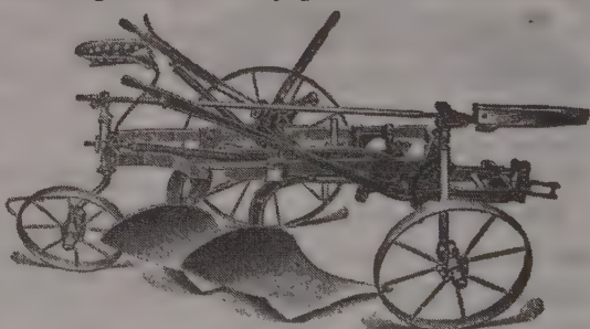
Fig. 113. A high-lift frame gang plow.
