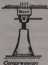
Fig. 256. A sketch illustrating a compressive stress.
