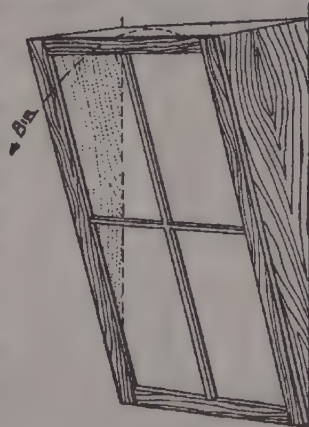
Fig. 321. A window arranged so as to allow air to enter with the least draft. It may be hinged at the bottom and made to close between the side pieces.
