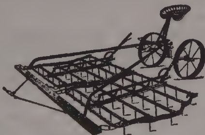
Fig. 119. A modern U-bar smoothing harrow with protected tooth bars. A harrow cart is attached.
