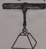
Tension Fig. 255. A sketch illustrating a tensile stress.
