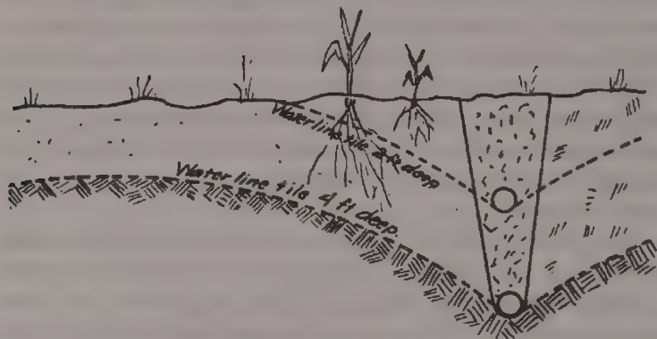
Fig. 44. Sketch showing how the ground water is lowered and the capacity of the soil as a reservoir increased by placing the tile deep.
