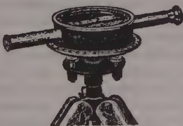
Fig. 24. An inexpensive farm level with horizontal circle for turning off angles.
