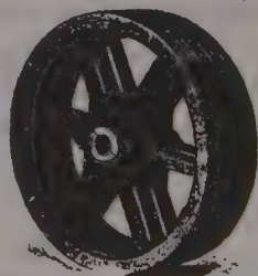
Fig. 202. A wooden pulley.
