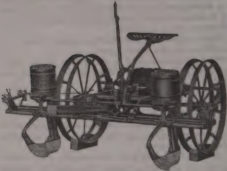
Fig. 142. A modern corn planter with long shoe furrow-openers, variable drop, and open wheels.
