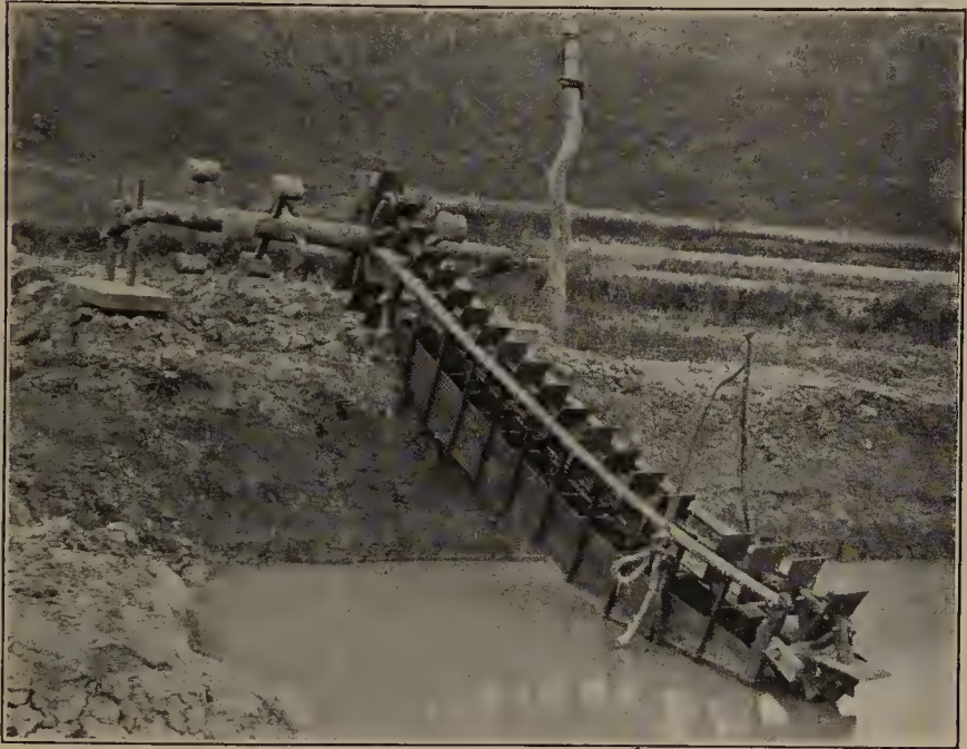
FIG. 153. — Three-man Chinese foot-power and wooden chain pump extensively used for irrigation in various parts of China.
